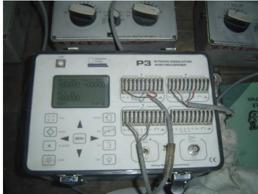
Picture 6. The Vishay P3 strain indicator used to indicate the strain gauge readings
