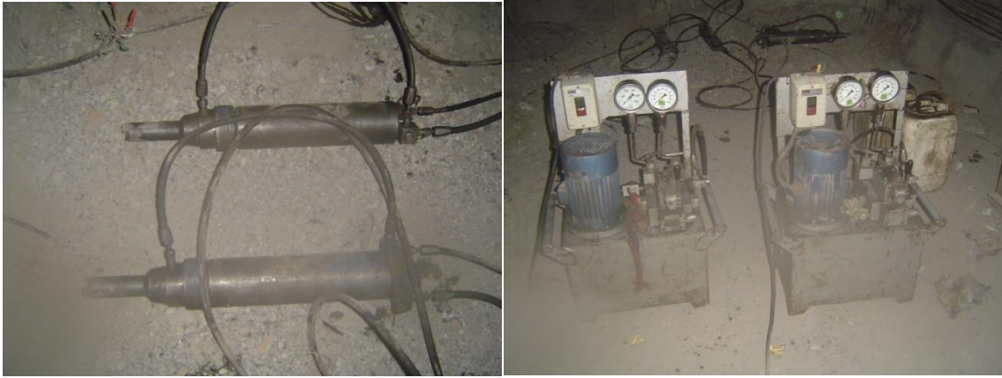
Picture set 2. The cable holding jack and the hydraulic pump system powered by electricity.
