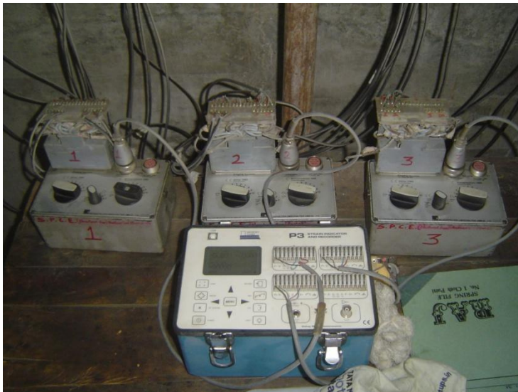
Picture 9. The whole setup including 3 Switcher Units and strain indicator used for strain measurements.
