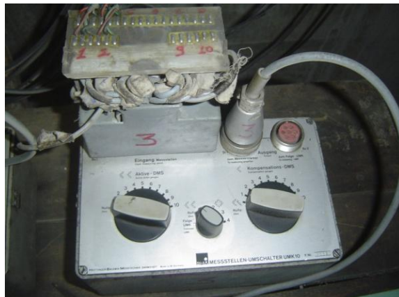
Picture 5. The HBM Germany made Selector Unit used for selecting the strain gauge.
