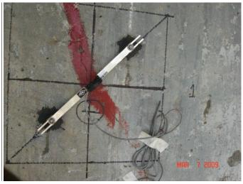
• To measure the change in frequency of vibration, before and after strengthening, of the girder piezoelectric accelerometers of B & K Denmark Make were mounted at the centre of the four girders on the bottom face in the mid span positions. Measurements were done with the help of standard loaded vehicle moving at constant velocity of 25 kmph.
