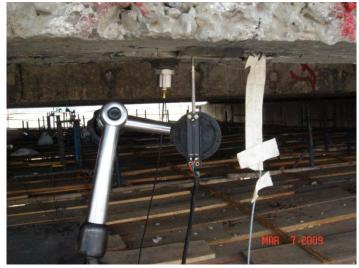
• To measure Flexural strains, before and after strengthening, foil type PL-60 TML Japan Make electrical strain gauges were mounted at the two girders(1 and 5) in all three spans. Readings were taken by using standard loaded vehicles positioned to induce bending moment.
