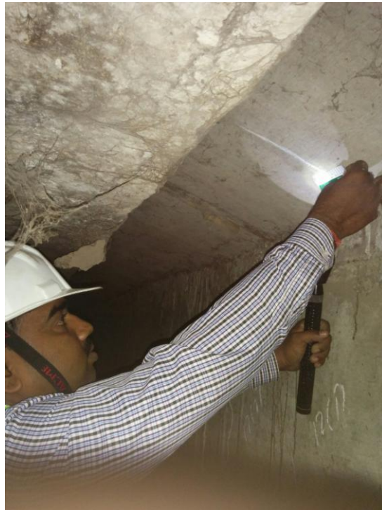
Fig 3.1 – Crack width Measurement card
