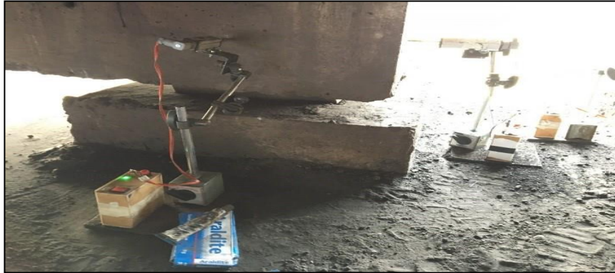
Fig 6: Placing of Linear Potentiometer
