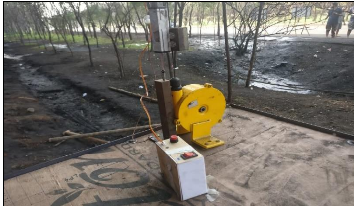
Fig 2: - Linear Potentiometer to find deflection.
